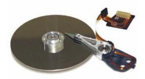
The information is stored in circular patterns on the disk and the computer measures the location of the rings and the spatial resolution is very high, so the location of the head to find data on the disk is extremely precise.
